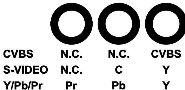
The recommended input level is 0.7-1V p-p. The input level shall not exceed 3V p-p, this may damage the unit.
