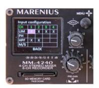
A comprehensive menu system offers full control of signal routing and input configuration, as well as for recording and time-code setup.
